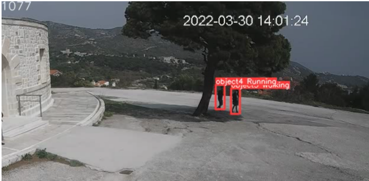
Figure 3-22 - Example of correct and false AR labeling for EfficientDet output
