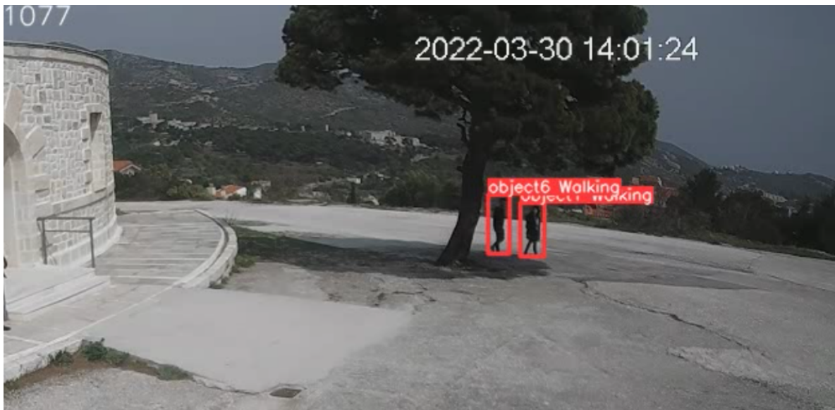
Figure 3-23 - Example of correct AR labeling for YOLO output
