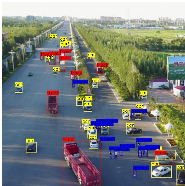
Figure 3-12 - Example of outdoor Object detection using YOLO v4
