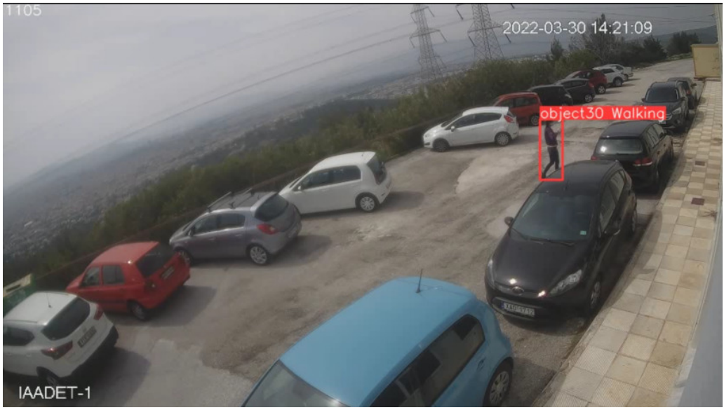
Figure 3-26 - Example of correct AR labeling for YOLO output
